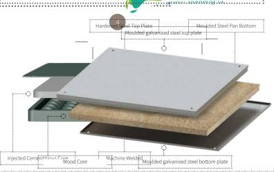
nel is screw fixed to the pedestal head at all
