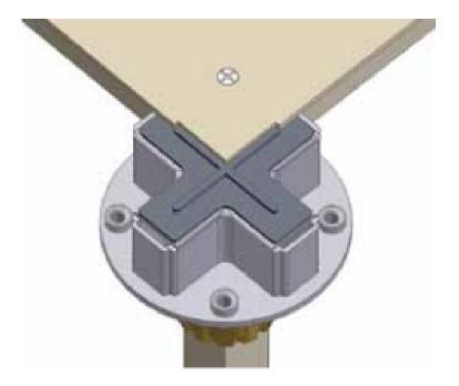
The built-in expansion joint and panel cut-out: is designed to keep the panels separated by 0.3mm at all times. This eliminates the the panels clicking or rubbing up against each other. Noise and sound from an underfoot feel has always been a contentious issue with raised access floors. The ASP patented designs have eliminated the issues making for a solid underfoot feel and making it feel like you're walking on a standard concrete deck.
